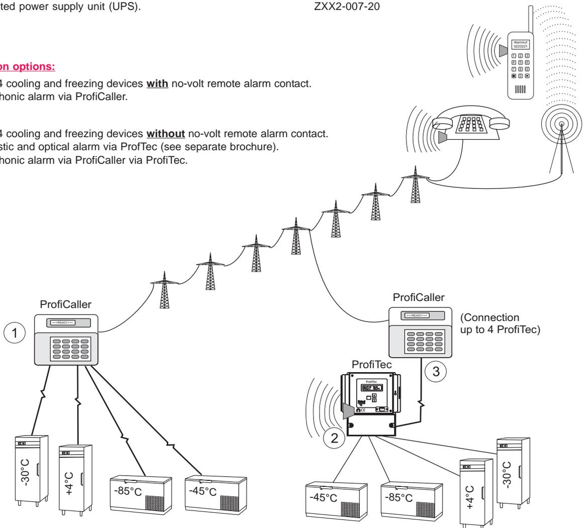
Chilling or freezing device **with** no-volt remote alarm contact
